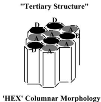
Figure 7 Scheme of a –DBAB– type of block copolymer "tertiary structure".
